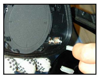
If your mirrors have the heater option, disconnect the heater wires at this time. Carefully remove the foam disc from the back of the mirror and set it aside.
